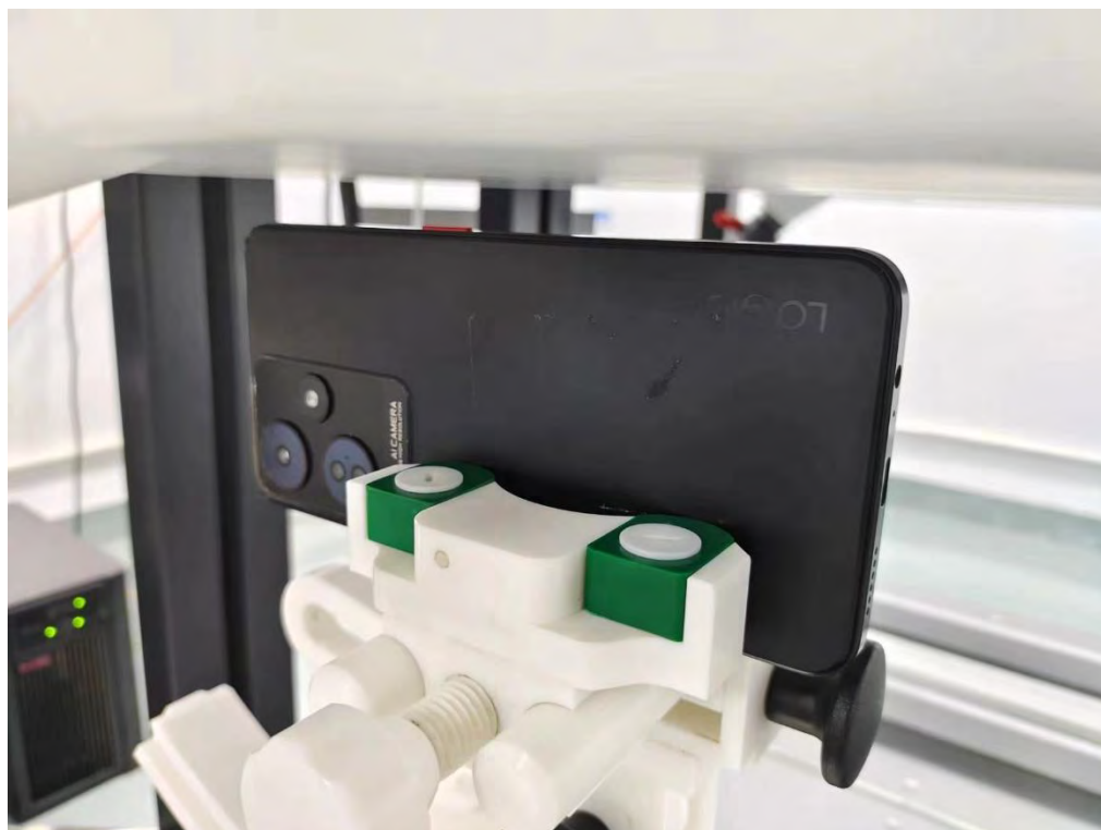
Body Left side (separation distance is 10mm)
