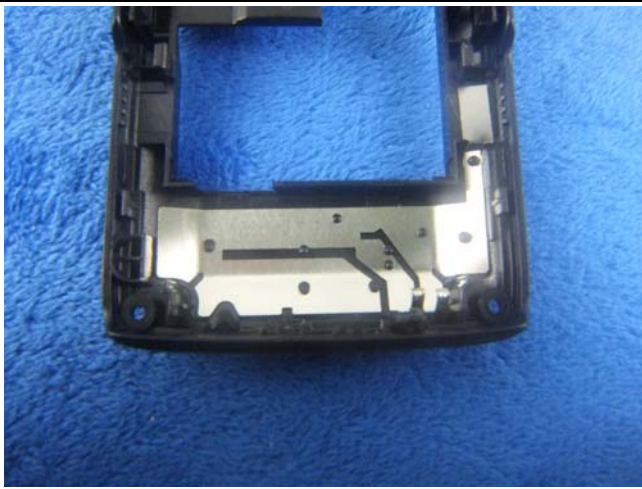
GSM Antenna View
