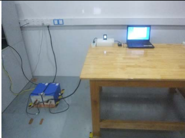
Conducted Emissions Test Setup – Front View
