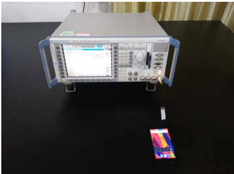
Photograph –2G&3G Conducted Test Setup
