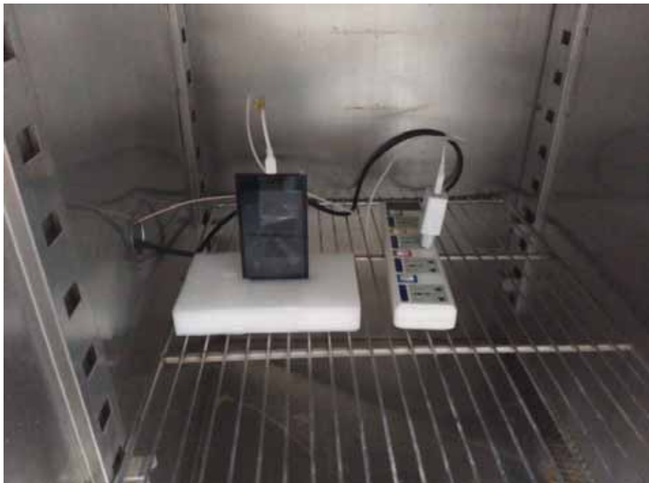
Photograph –2G&3G Conducted Test Setup
