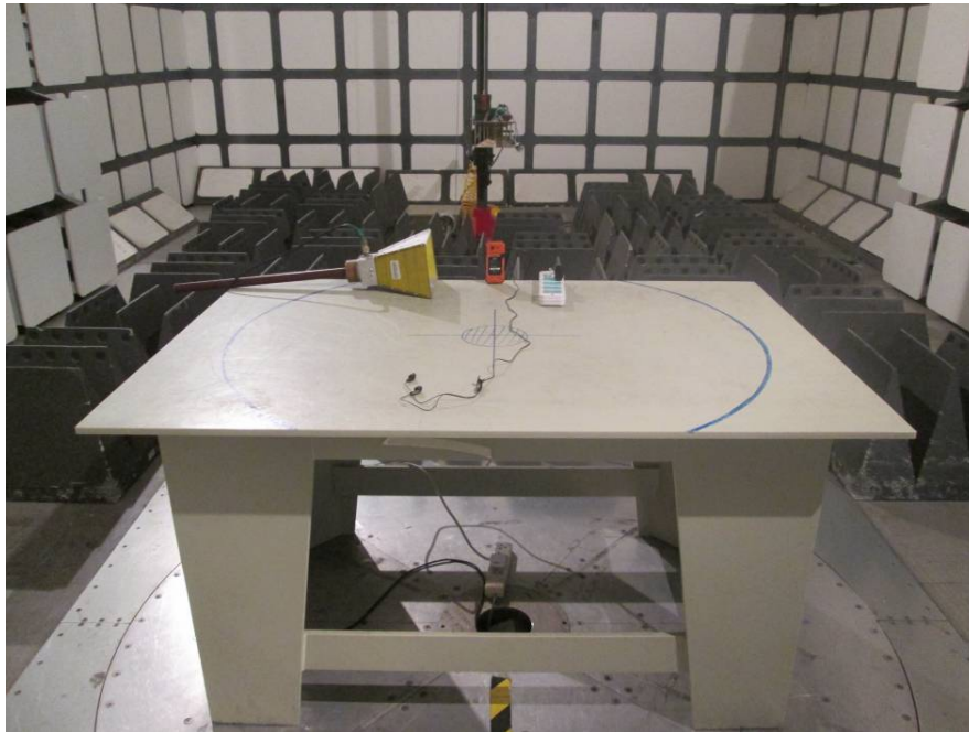
Radiated Emissions Front View (1-25 GHz)
