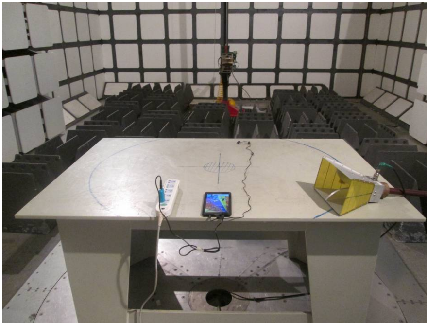
Radiated Emissions Rear View (Above 1GHz)
