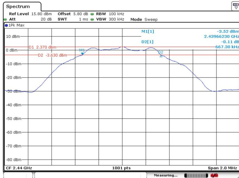
6 dB Bandwidth Plot on Channel 19
