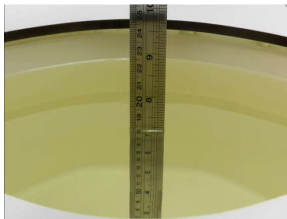
Fig 10.2 Photo of Liquid Height for Body SAR
