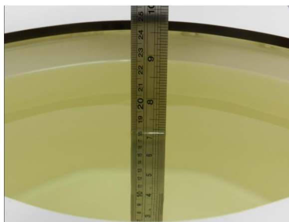
Fig 10.2 Photo of Liquid Height for Body SAR
