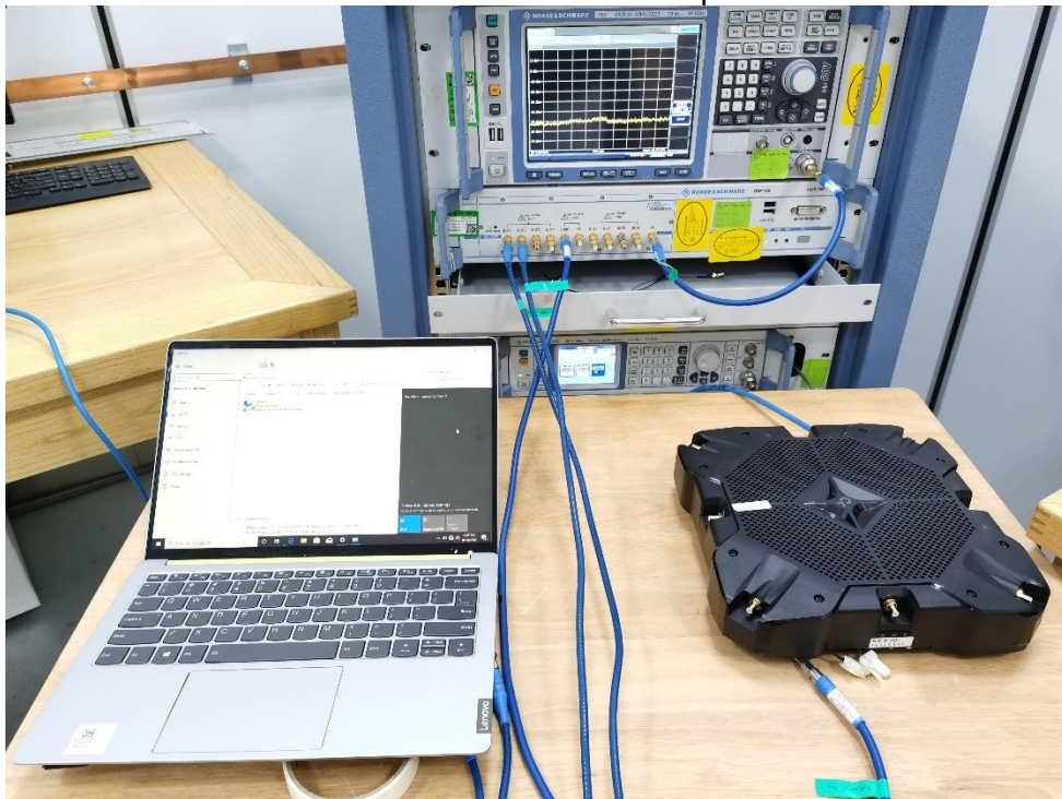
DFS Measurement Setup
