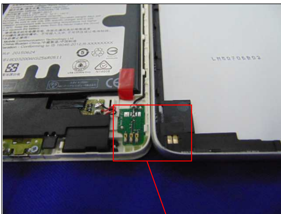
(Bottom) WWAN Main Antenna
