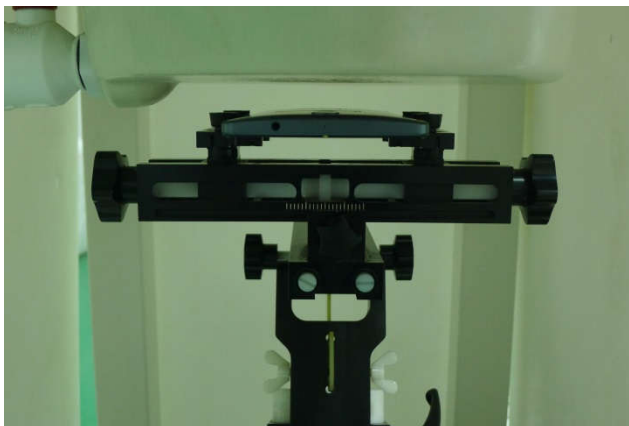
Back, Test Separation 15 mm
