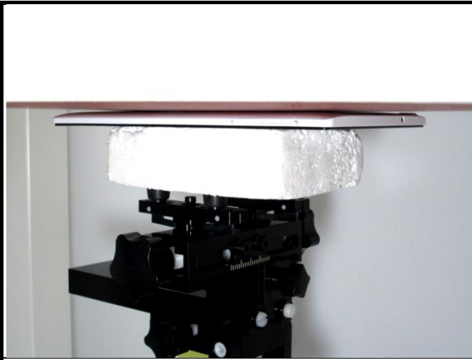
Rear Face of EUT with 0 mm Gap
