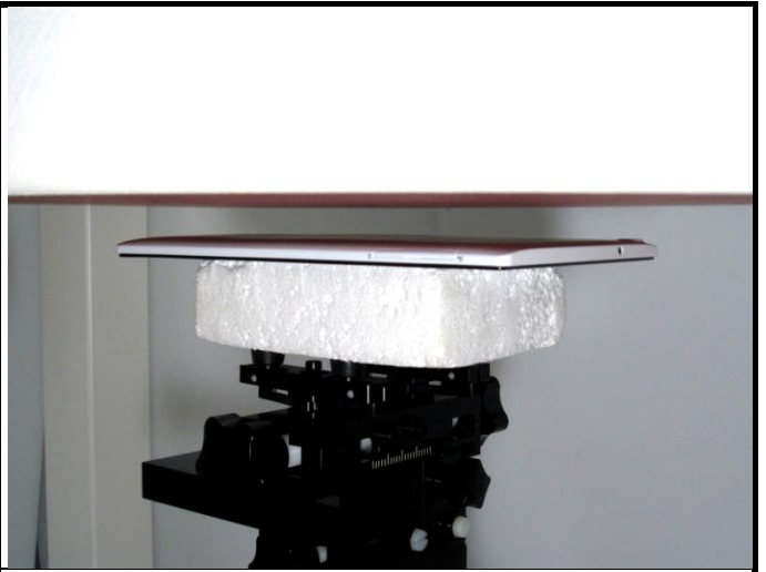
Rear Face of EUT with 13 mm Gap
