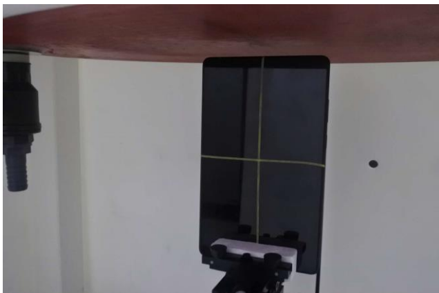
Edge 1 of EUT with Phantom 12 mm Gap
