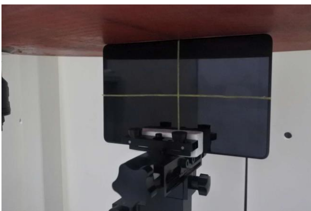
Edge 4 of EUT with Phantom 0 mm Gap
