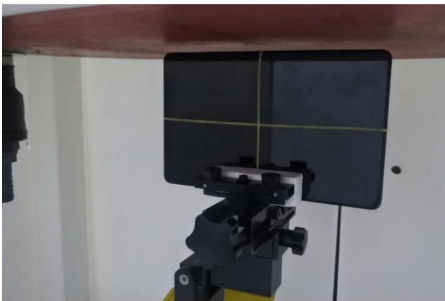
Edge 2 of EUT with Phantom 5 mm Gap
