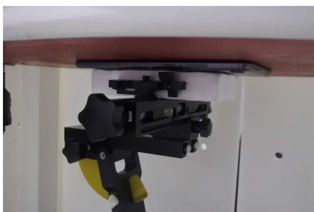
Bottom Face of EUT with Phantom 0 mm Gap
