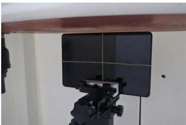
Edge 4 of EUT with Phantom 10 mm Gap
