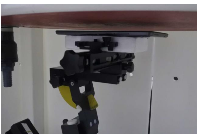
Bottom Face of EUT with Phantom 13 mm Gap
