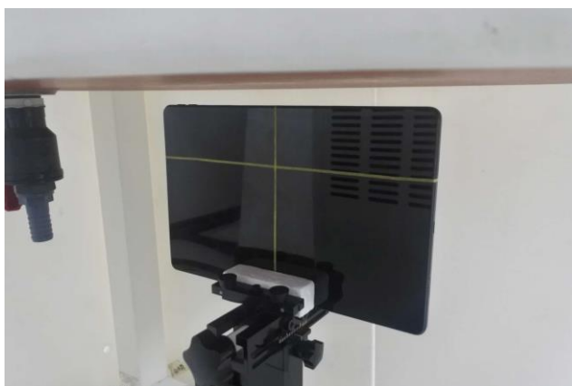
Edge 1 of EUT with Phantom 23 mm Gap (Sensor off) for Antenna 1
