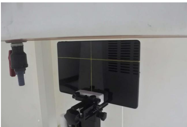
Edge 1 of EUT with Phantom 8 mm Gap (Sensor off) for Antenna 3
