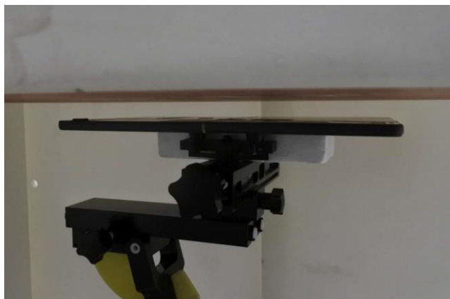
Bottom Face of EUT with Phantom 18 mm Gap (Sensor off) for Antenna 2
