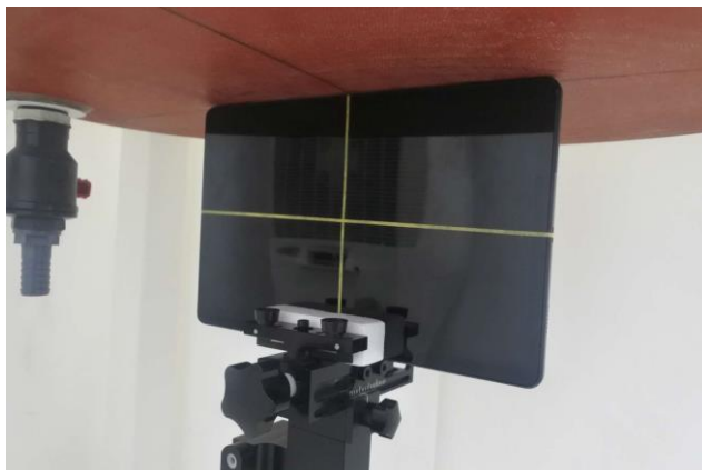
Edge 1 of EUT with Phantom 0 mm Gap
