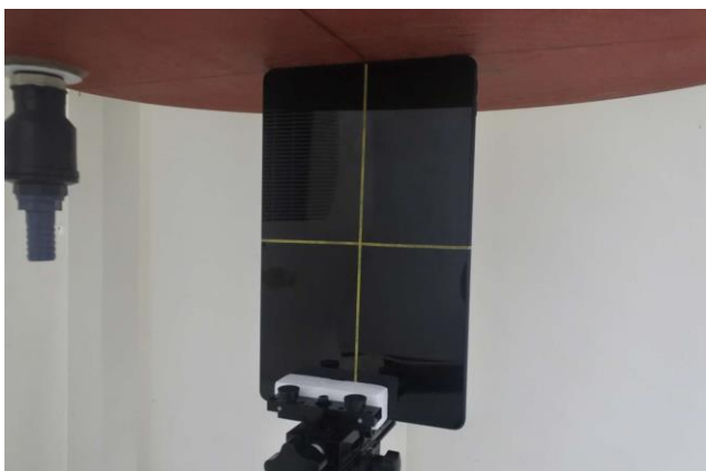
Edge 4 of EUT with Phantom 0 mm Gap
