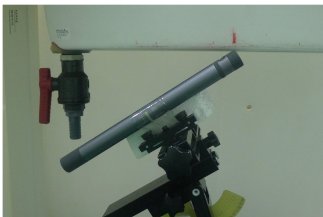
Bottom Face Edge 1_35 Degree, Test Separation 1 cm
