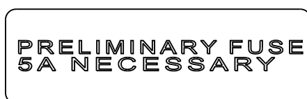
Figure 2-8 Preliminary Fuse Label
