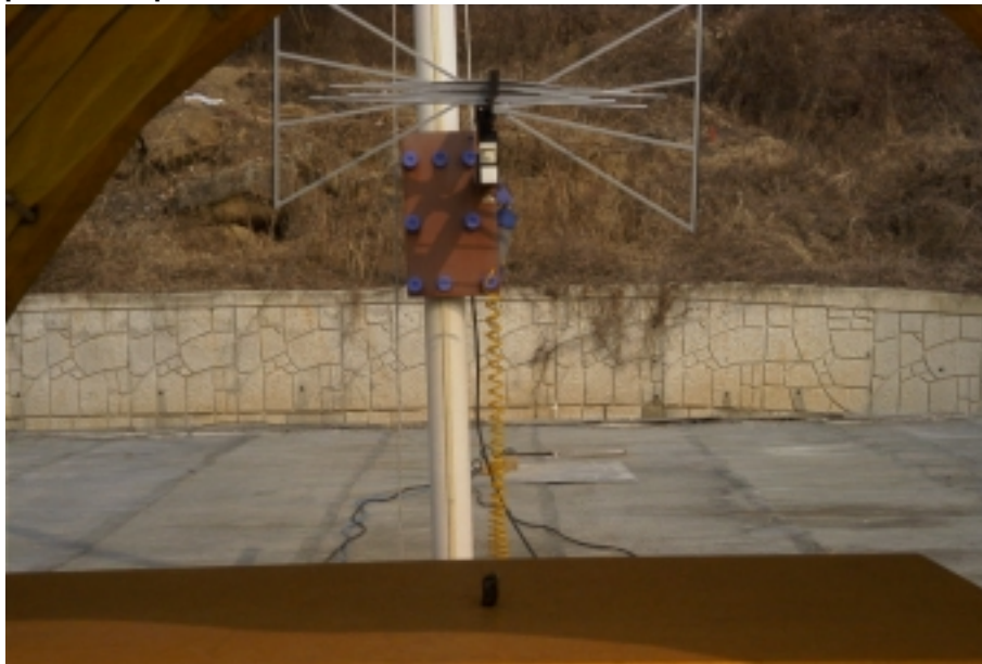
Photograph 1 : Setup for radiated Emissions
