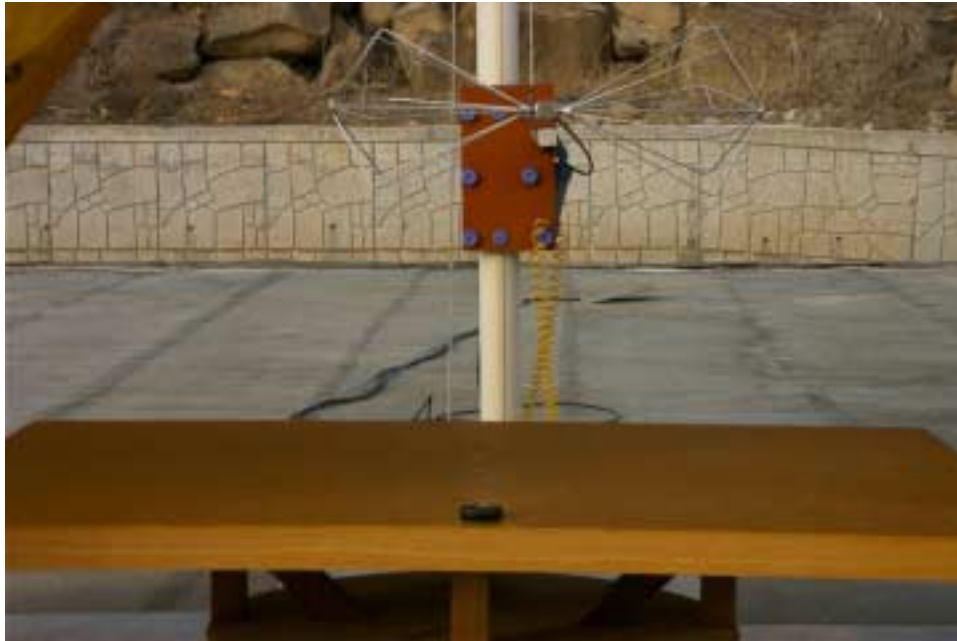
Photograph 1 : Setup for radiated Emissions
