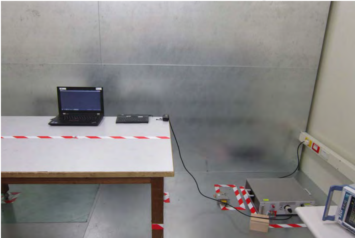
AC Power-line Conducted Emission Set up Photo
