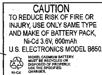
BATTERY CAUTION LABEL (TO BE PLACED INSIDE BATTERY COMPARTMENT)
