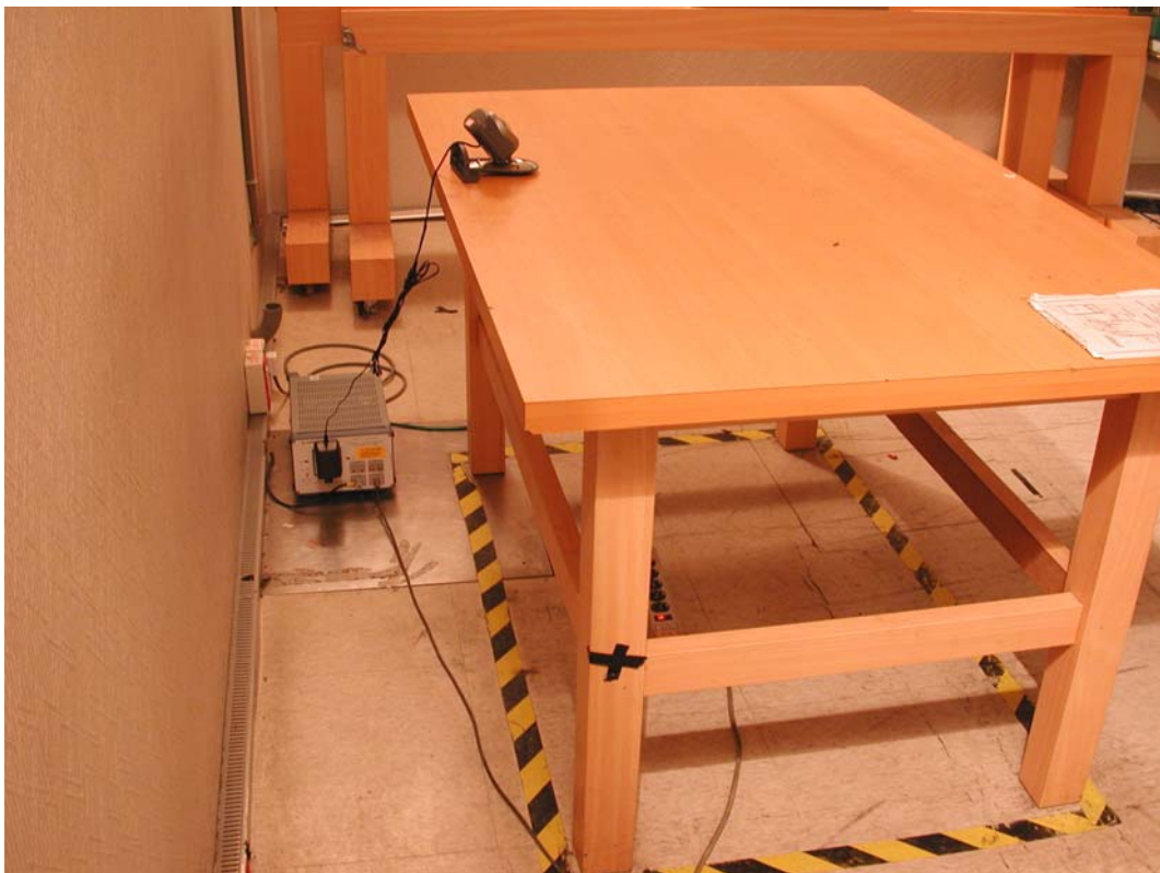
Back View of Conducted Test (Adapter: R410905)
