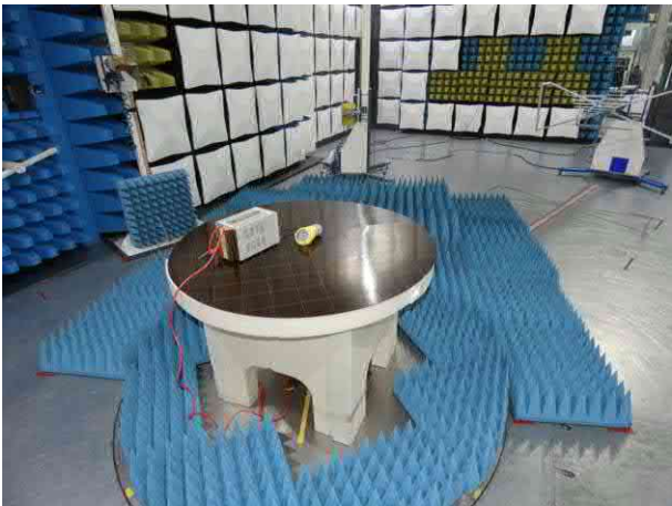
Photo 8-10: Test setup for radiated measurements (semi anechoic chamber, CFR 47 Part 15, Subpart B)
