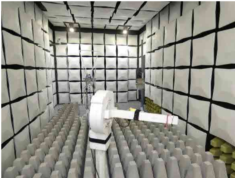
Photo 6-7: Test setup for radiated measurements (fully anechoic chamber, CFR 47 Part 15, Subpart B)
