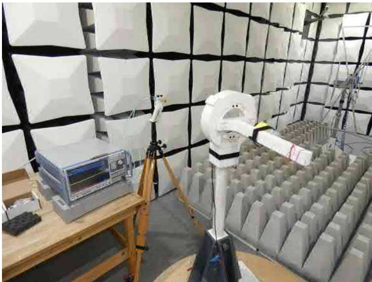
Photo 2-3: Test setup for radiated measurements (fully anechoic chamber, CFR 47 Part 15, Subpart C, §256)
