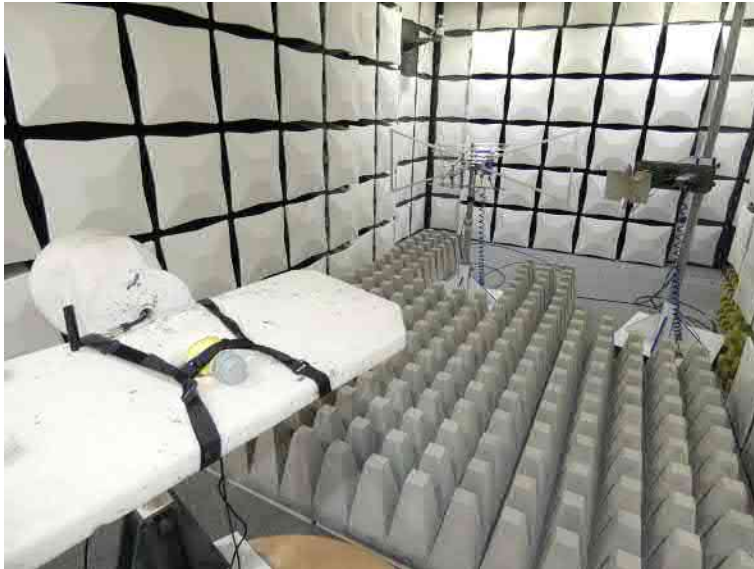
Photo 1: Test setup for radiated measurements (fully anechoic chamber, CFR 47 Part 15, Subpart C, §247)
