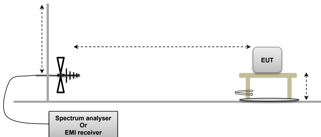
Test setup of Field strength within the band 13.110-14.010MHz in OATS
