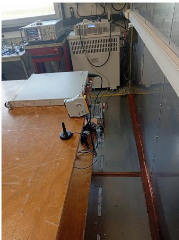
Photo of AC Power Line Conducted Emissions ( direct AC power)
