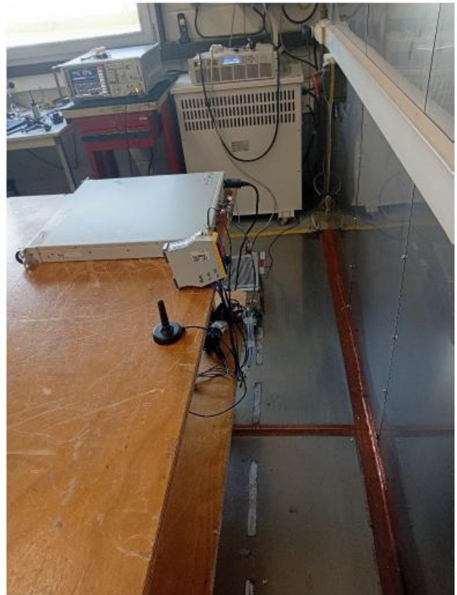
Photo of AC Power Line Conducted Emissions with Power supply for DC supply mode
