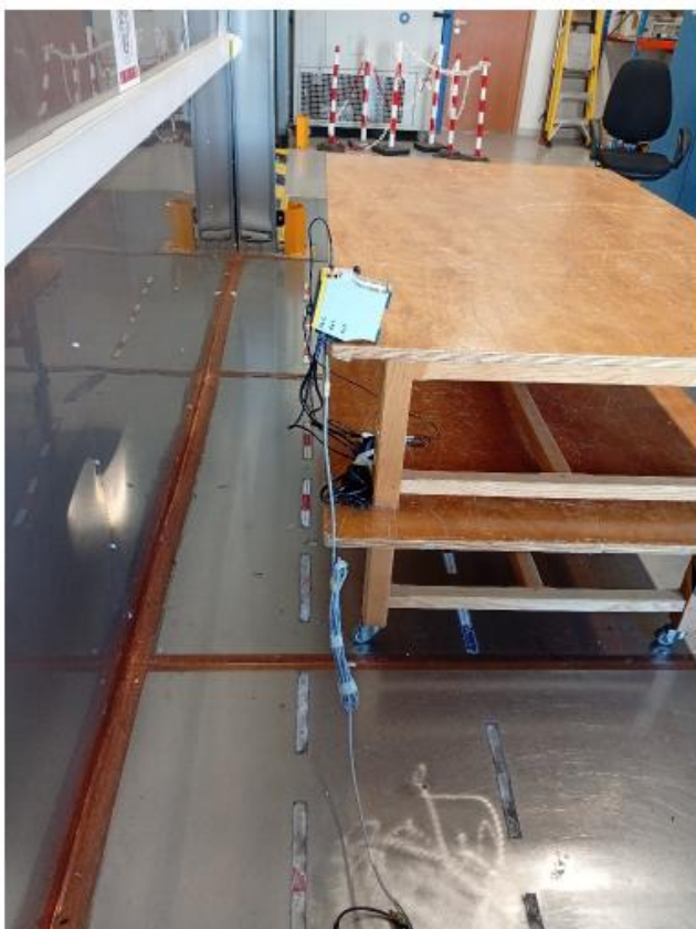
Photo of AC Power Line Conducted Emissions ( direct AC power)
