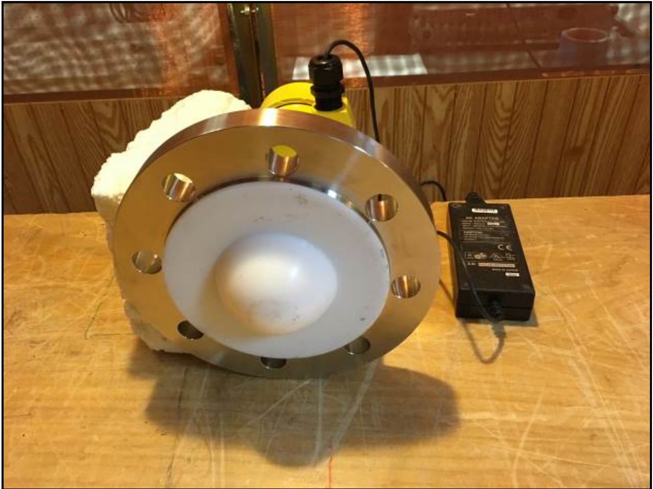
Photograph 7: AC Conducted Emissions – Front View - TC #2
