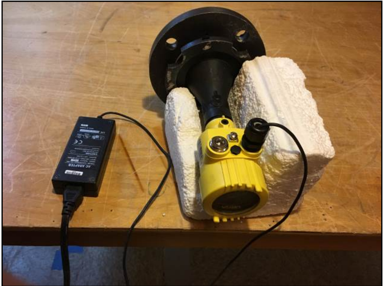
Photograph 6: AC Conducted Emissions - Rear View – TC #1
