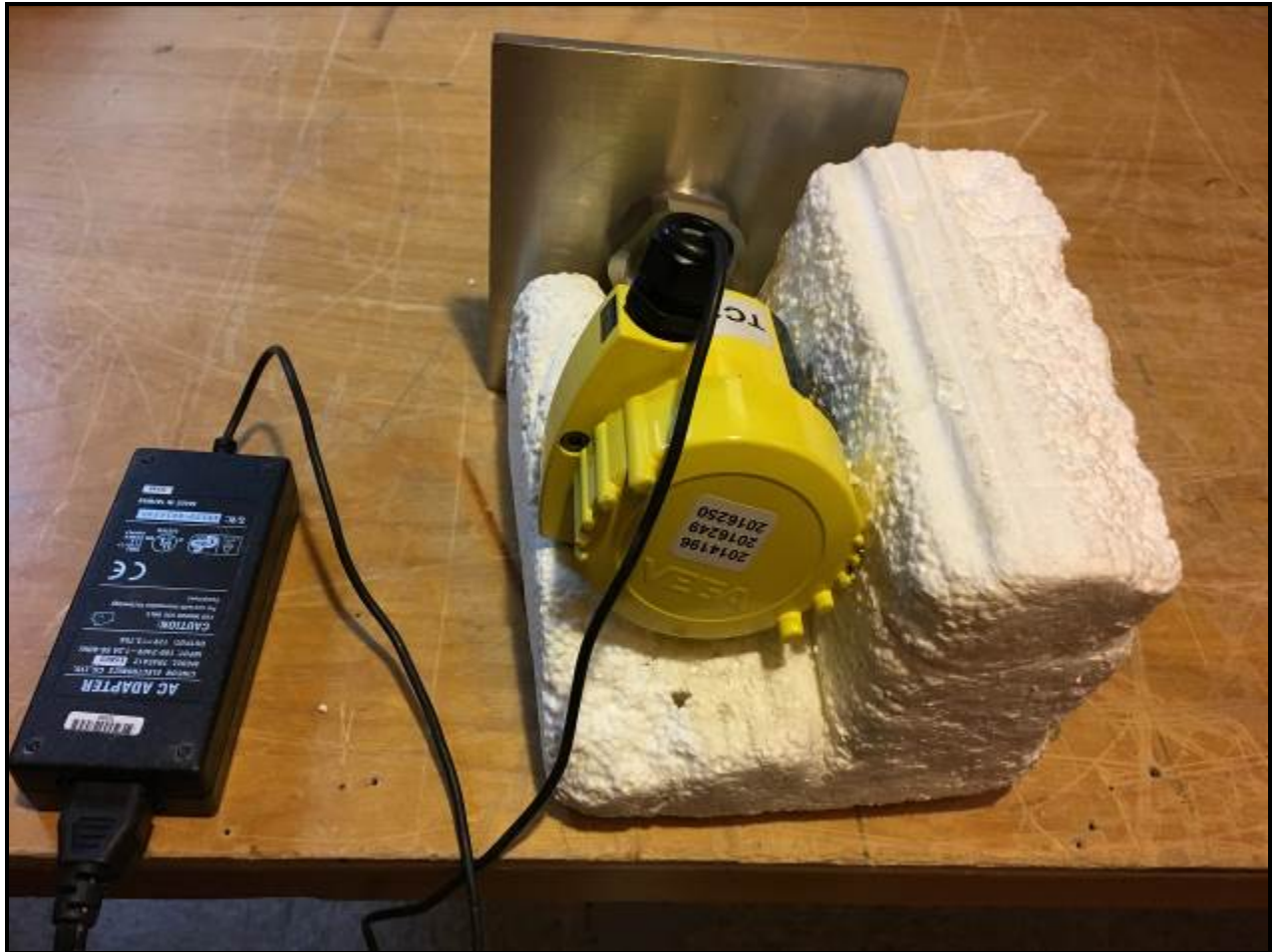
Photograph 10: AC Conducted Emissions - Rear View – TC #3
