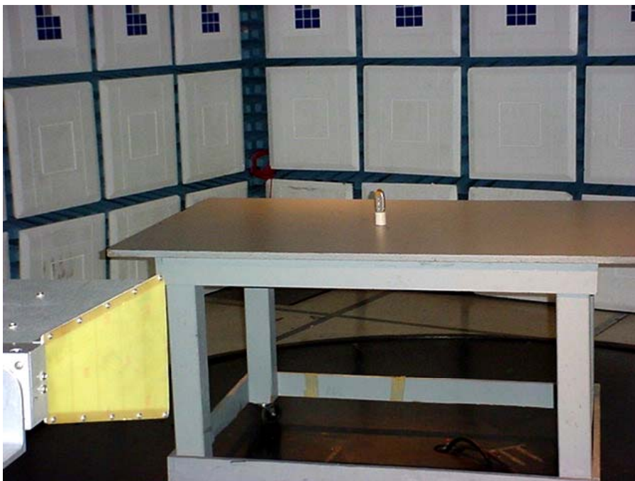
Radiated Emissions in Restricted Bands Test Set-Up
