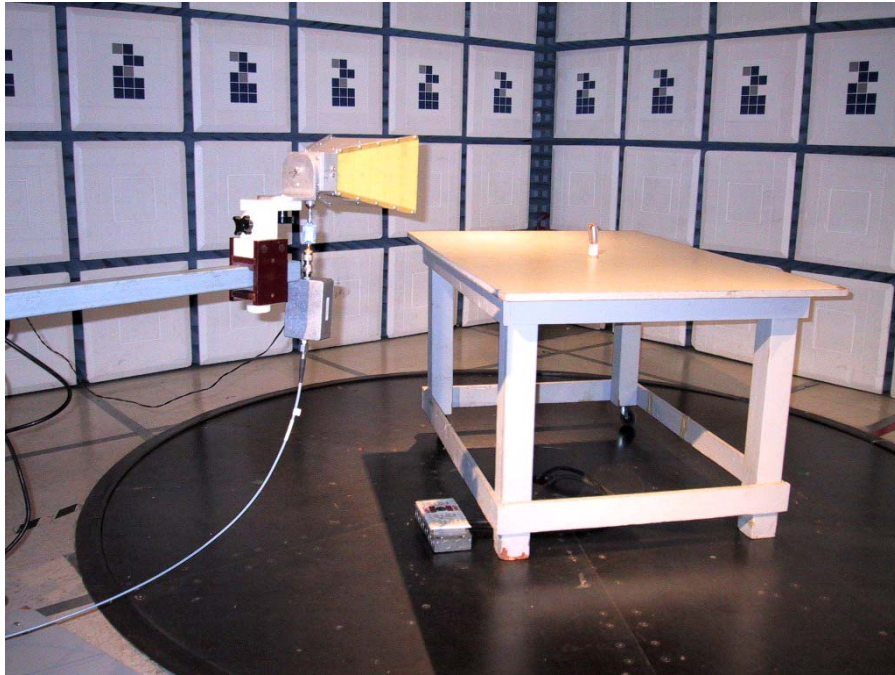
Radiated Emissions in Restricted Bands Test Set-Up
