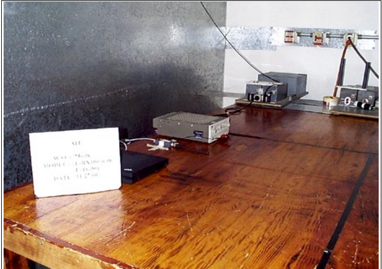
Conducted Emissions - Front View of Receiver
