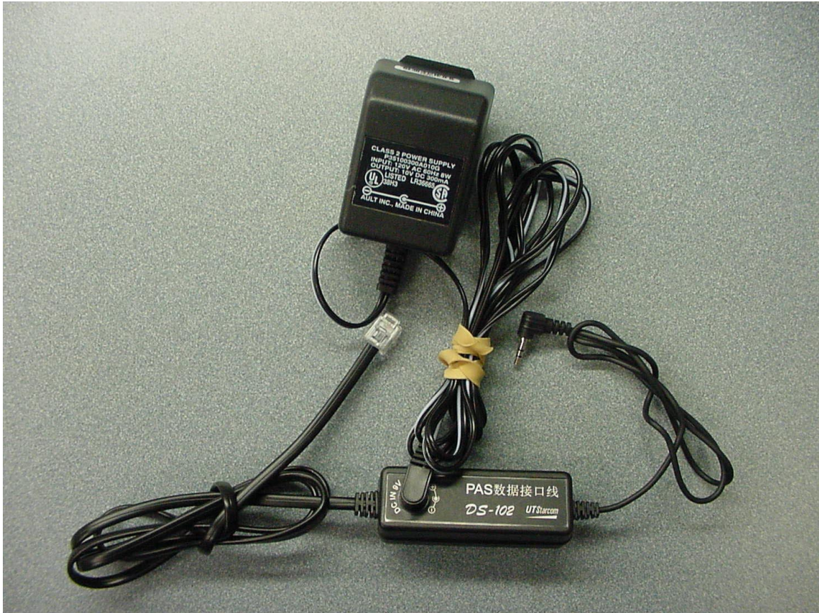
PHOTOGRAPH 37: DATA TRANSFER CABLE WITH POWER SUPPLY
