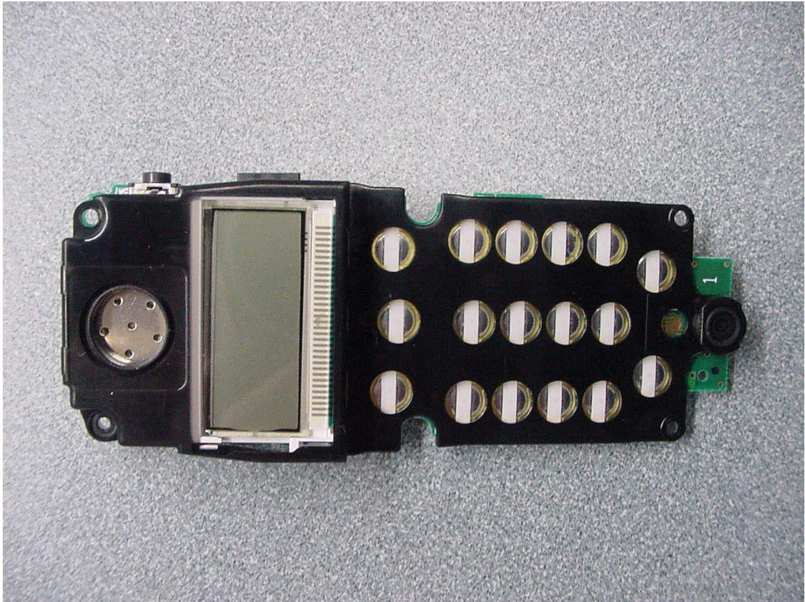
PHOTOGRAPH 19: FRONT OF PCB WITH PLASTIC HOLDDOWN
