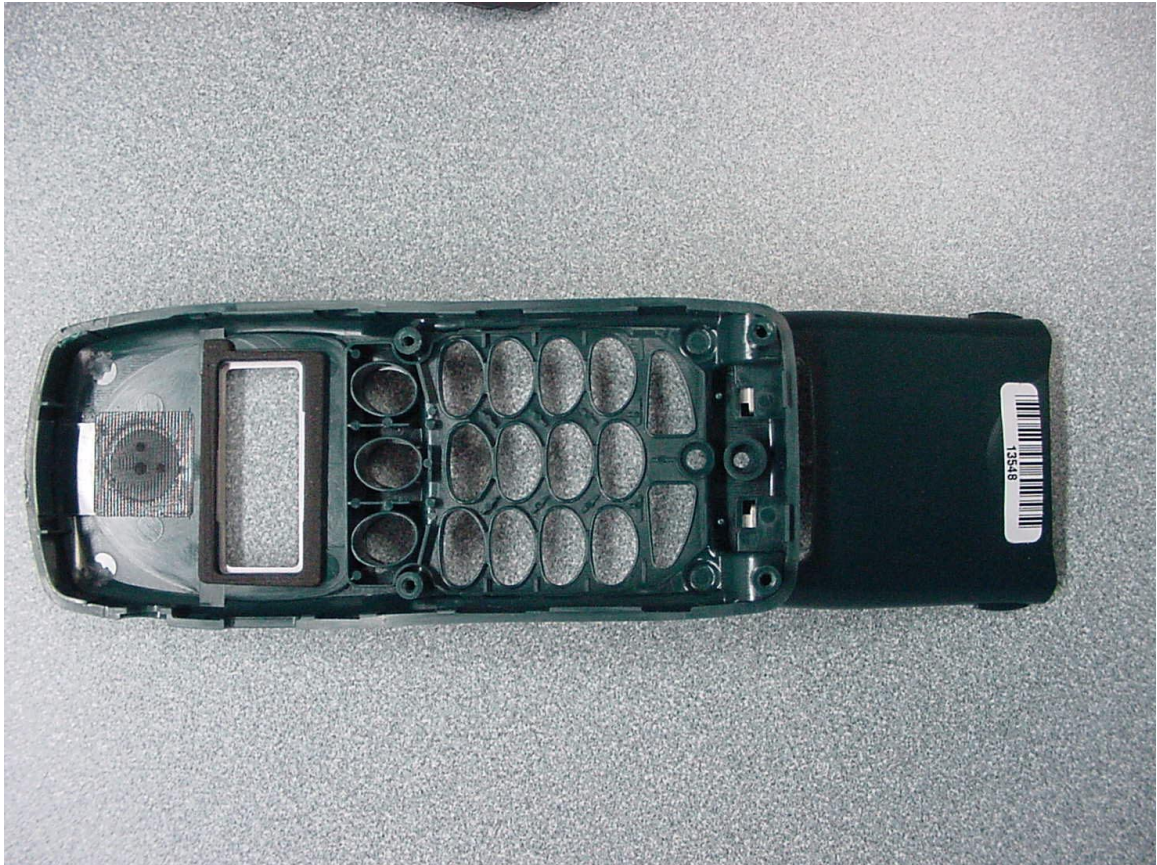
PHOTOGRAPH 13: BACK OF FRONT COVER WITH KEYPAD REMOVED
