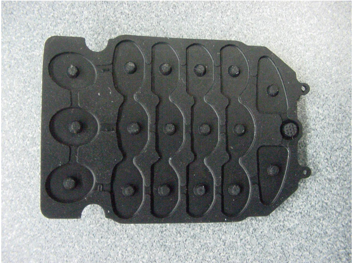
PHOTOGRAPH 12: BACK OF KEYPAD
