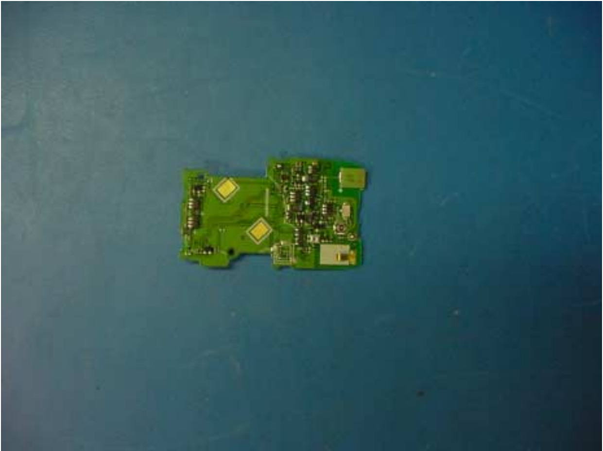
PHOTOGRAPH 14: SECONDARY REAR WITHOUT SHIELDS
