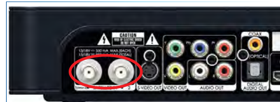
Check Satellite (SAT-IN) Connections
