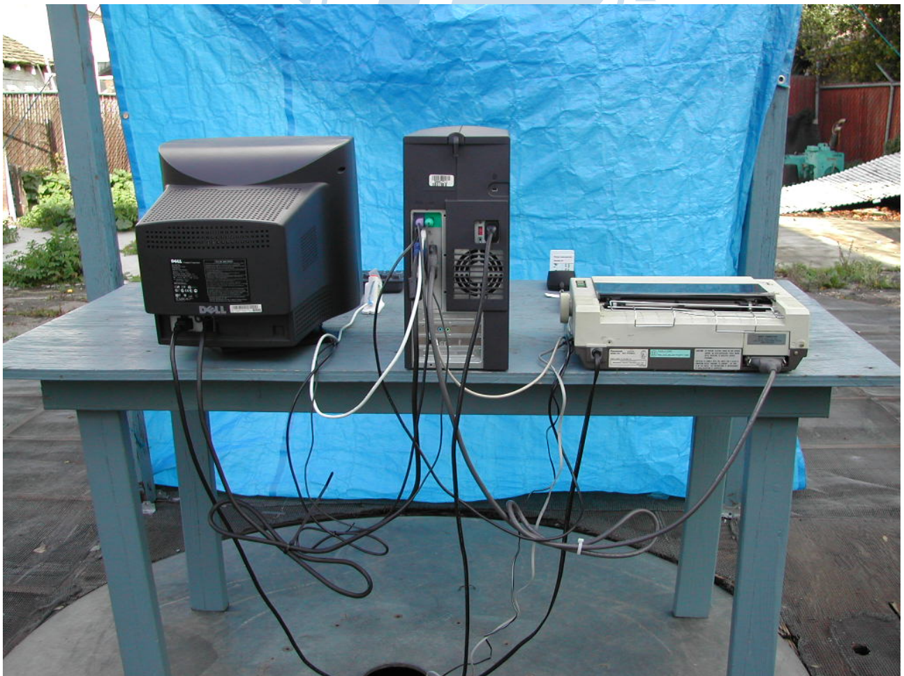
FIGURE 2: PLI Photograph Number 5346C2934SJ-06 illustrates the rear view of the Equipment Under Test with all peripherals attached in Test Configuration #1 . The "open field" radiated and the "screen room" conducted Radio Frequency Interference / Electromagnetic Interference test programs utilized this equipment and cable configuration.
