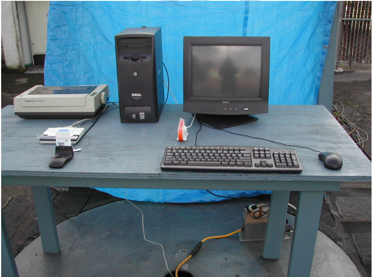
FIGURE 3: PLI Photograph Number 5346C2934SJ-08 illustrates the front view of the Equipment Under Test with all peripherals attached in conducted Electromagnetic Interference Test Configuration #1 .
