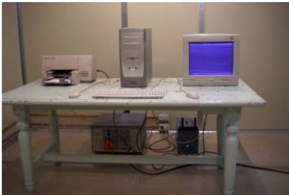
Photograph 2 : Setup for Conducted Emissions
