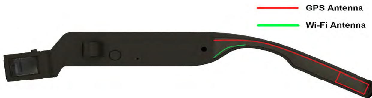
Antenna location of the glasses (Inside view)
