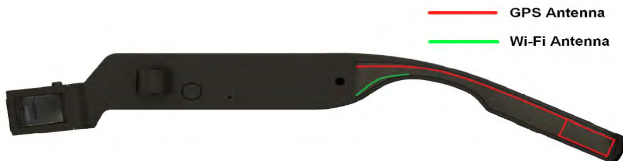
Fig.8 Antenna position of EUT (Inside view) - End of Report -
