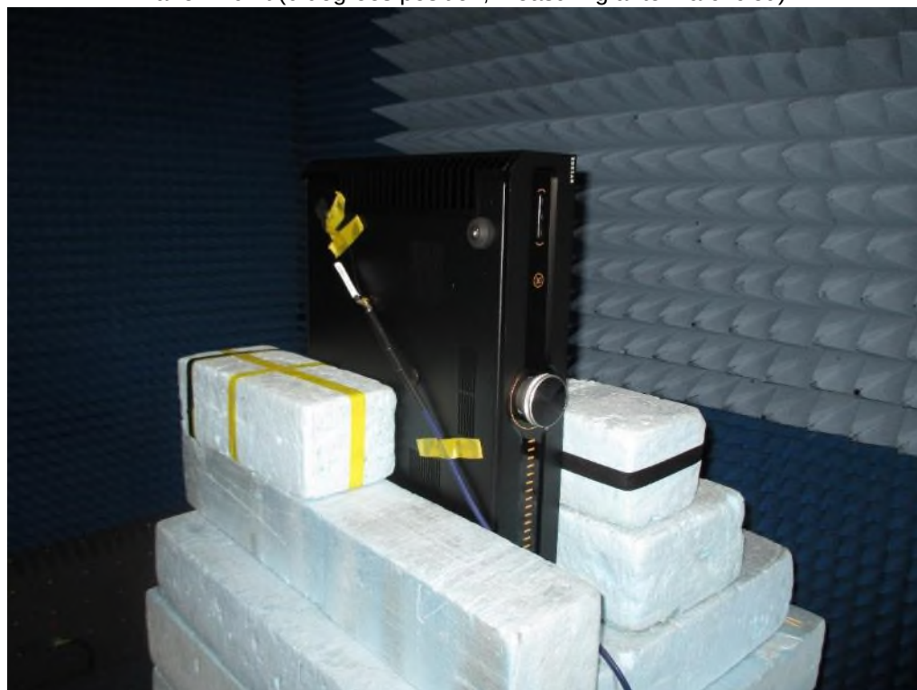
Caspian 4G amplifier orientation for ESP32 antenna tests only.
