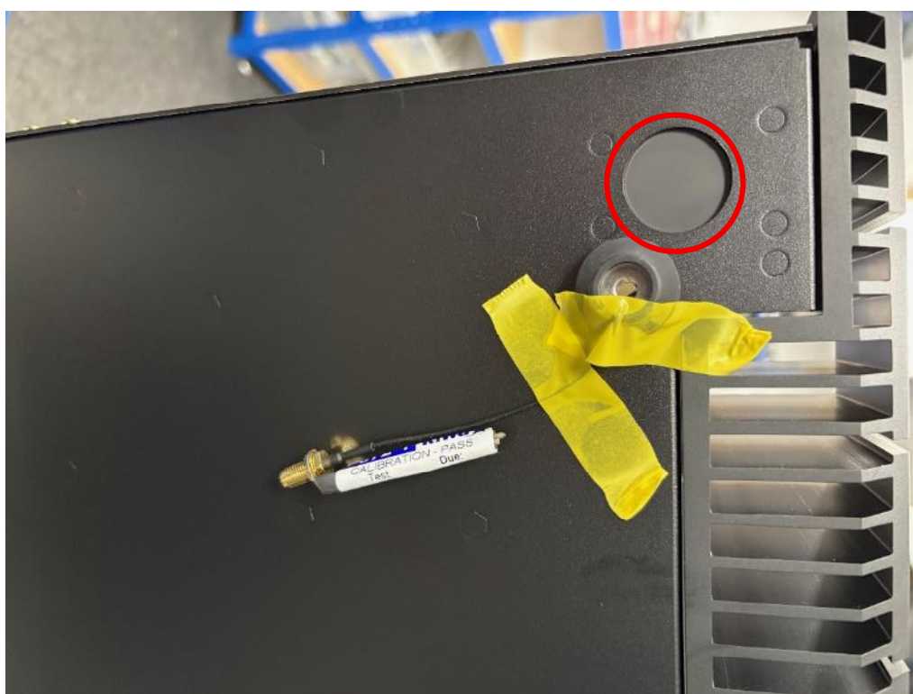
BLE/2.4 WiFi antenna location (circled) - underside of chassis. (Antenna 1)
