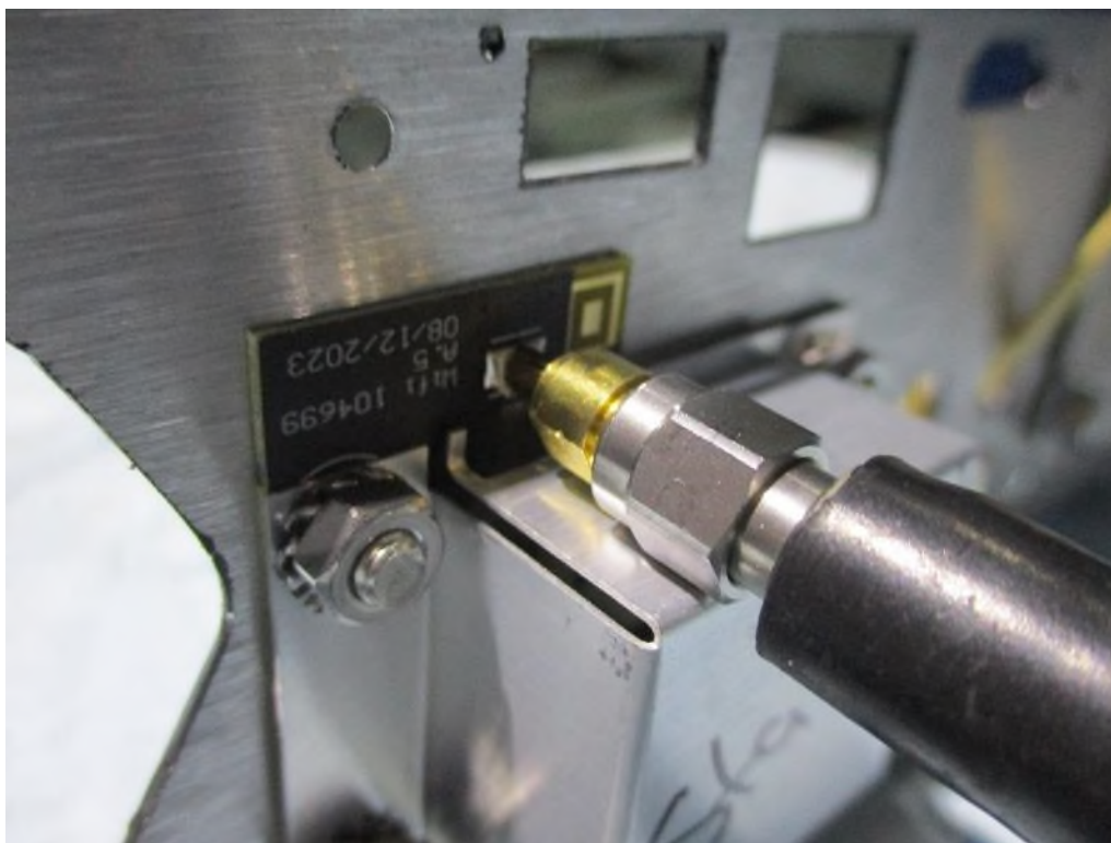
Antenna 2 - 'Standard' antenna port (in BTC location).
