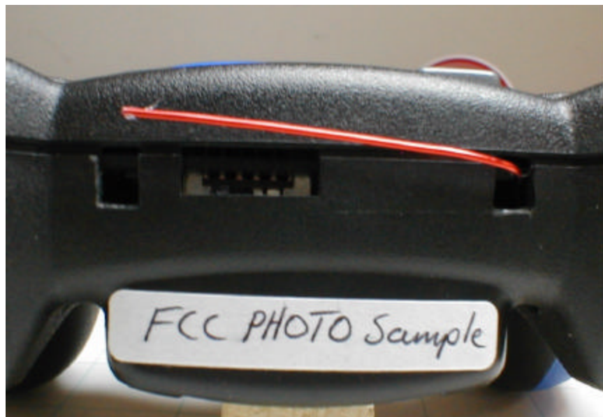
Antenna Cover Removed
