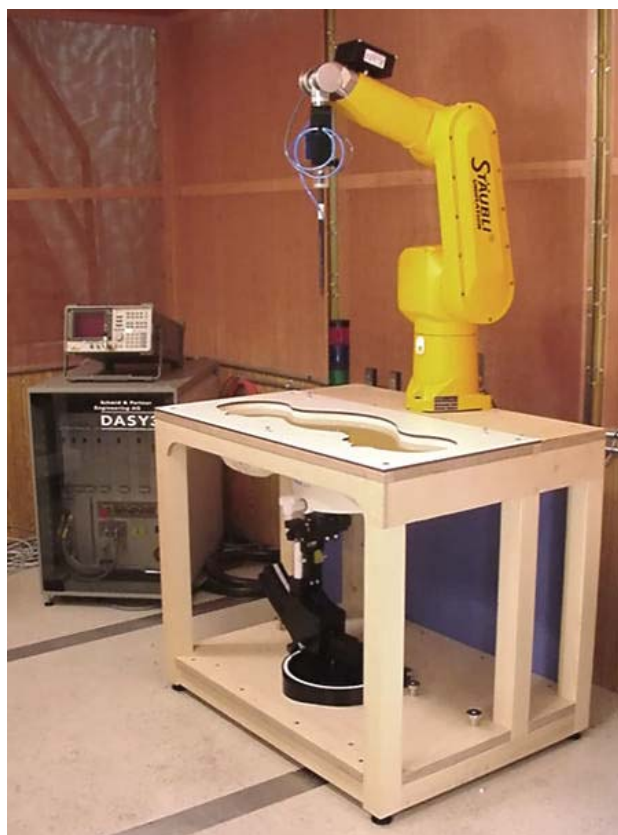
DASY3 SAR Measurement System with SAM Phantom
