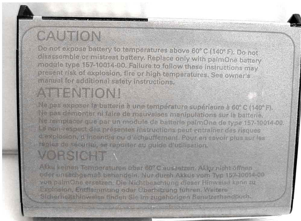
Lithium-ion Battery (P/N: 157-10014-00)
