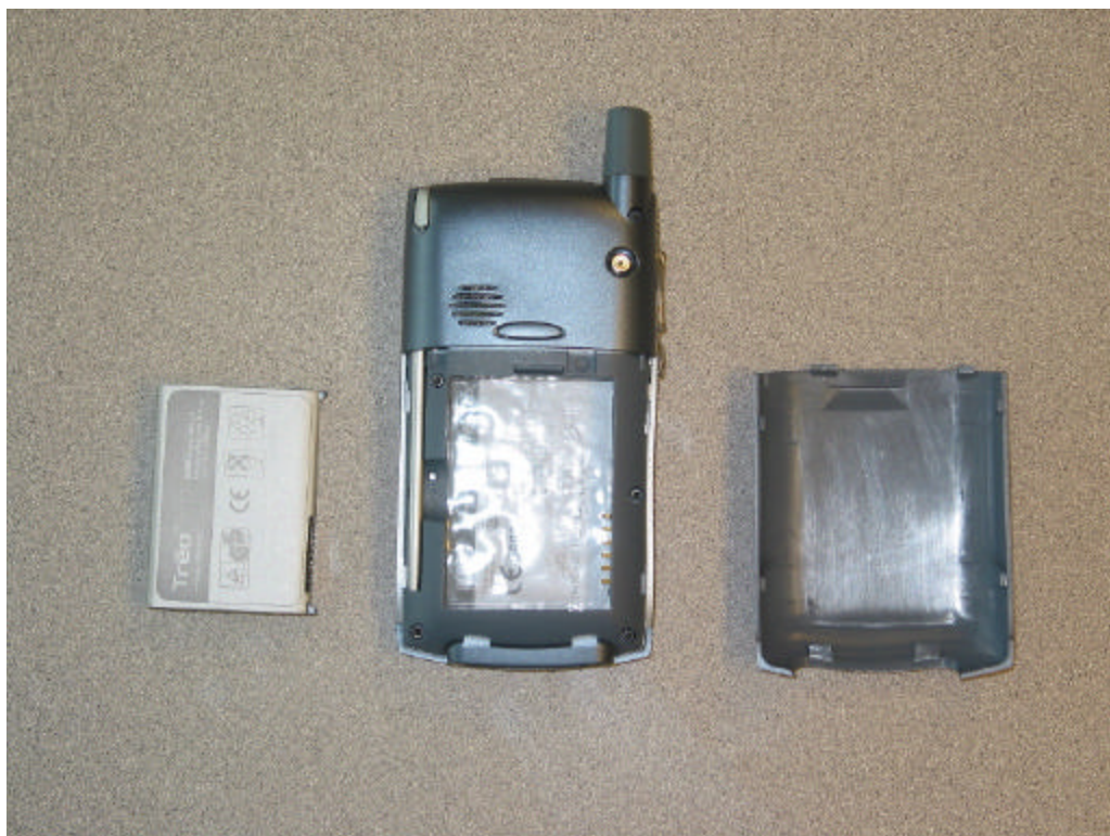
Battery and cover removed
