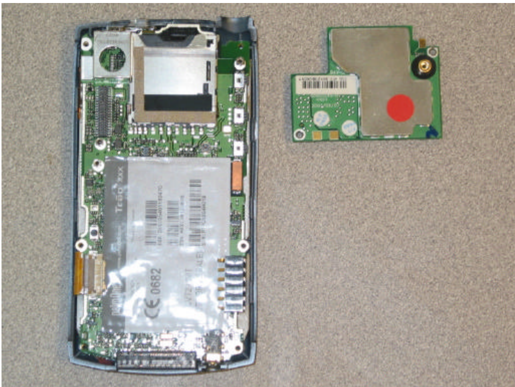
RF Module Removed
