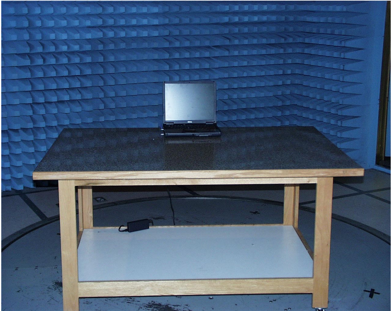
Front View of Radiated Test Setup
