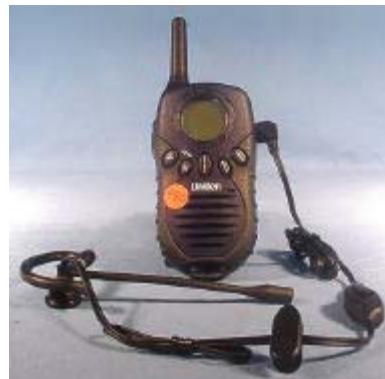
EUT with Speaker-Microphone
