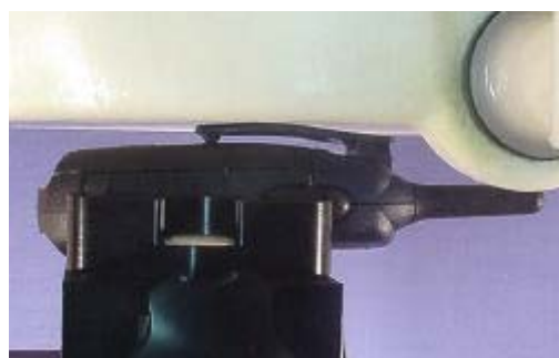
Body-worn SAR Test Setup 0.7cm Belt-Clip Separation
