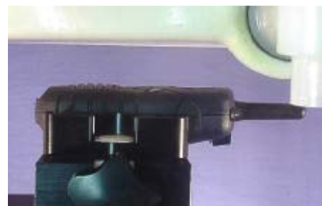
Face-Held SAR Test Setup 2.5cm Separation Distance
