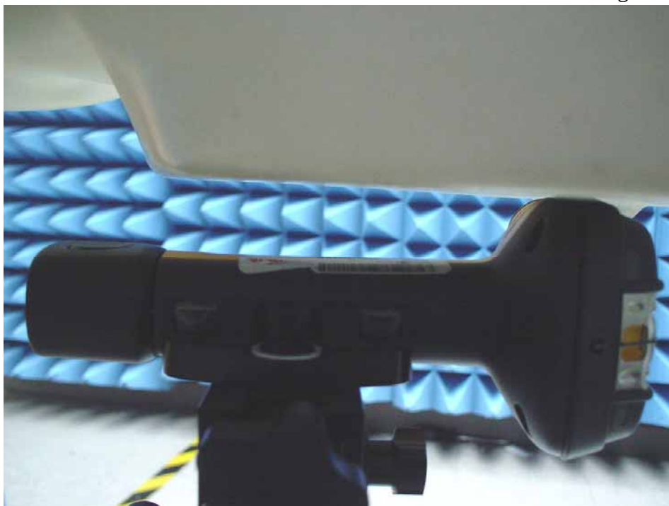
Fig.5 Photo of the EUT Left-side contact to the Flat phantom, Spacing between EUT and phantom –In contact (0mm)
