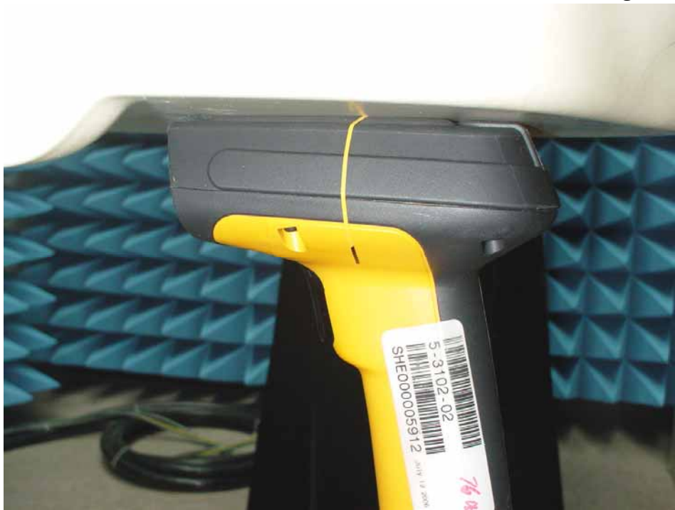
Fig.3 Photo of the EUT face-on contact to the Flat phantom, Spacing between EUT and phantom –In contact (0mm)
