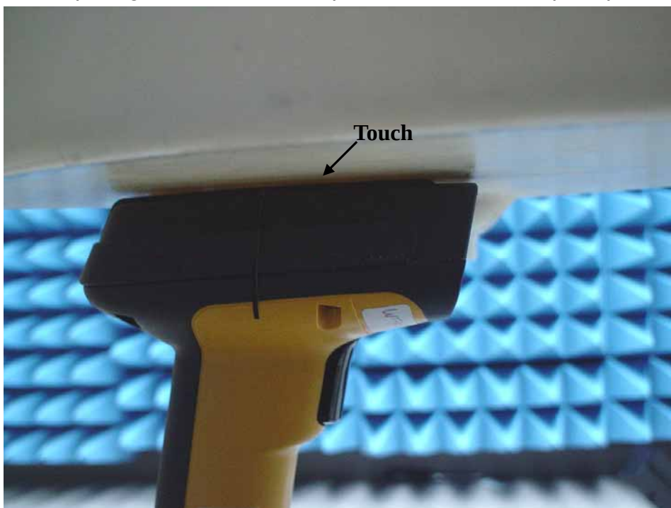
Fig.4 Photo of the EUT face-on contact to the Flat phantom, Spacing between EUT and phantom –In contact (0mm)
