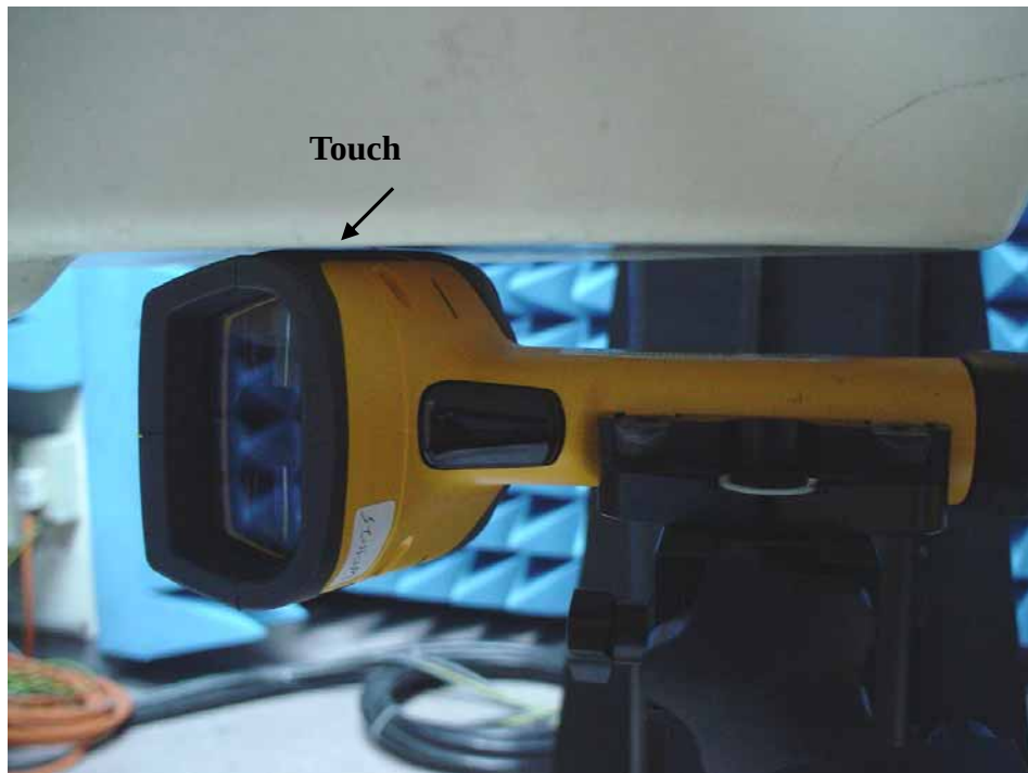
Fig.6 Photo of the EUT Left-side contact to the Flat phantom, Spacing between EUT and phantom –In contact (0mm)
