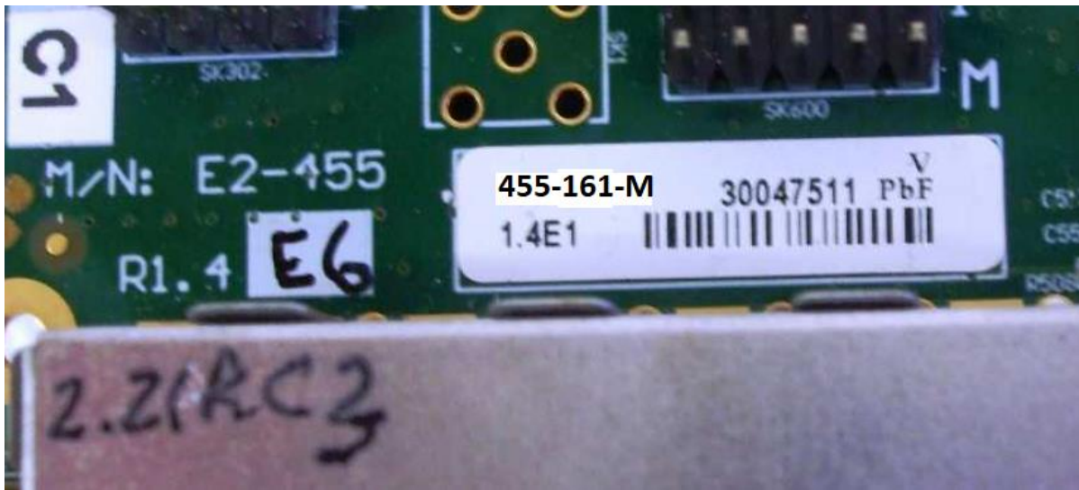
Card to provide DC and RS232 connections to the DUT
