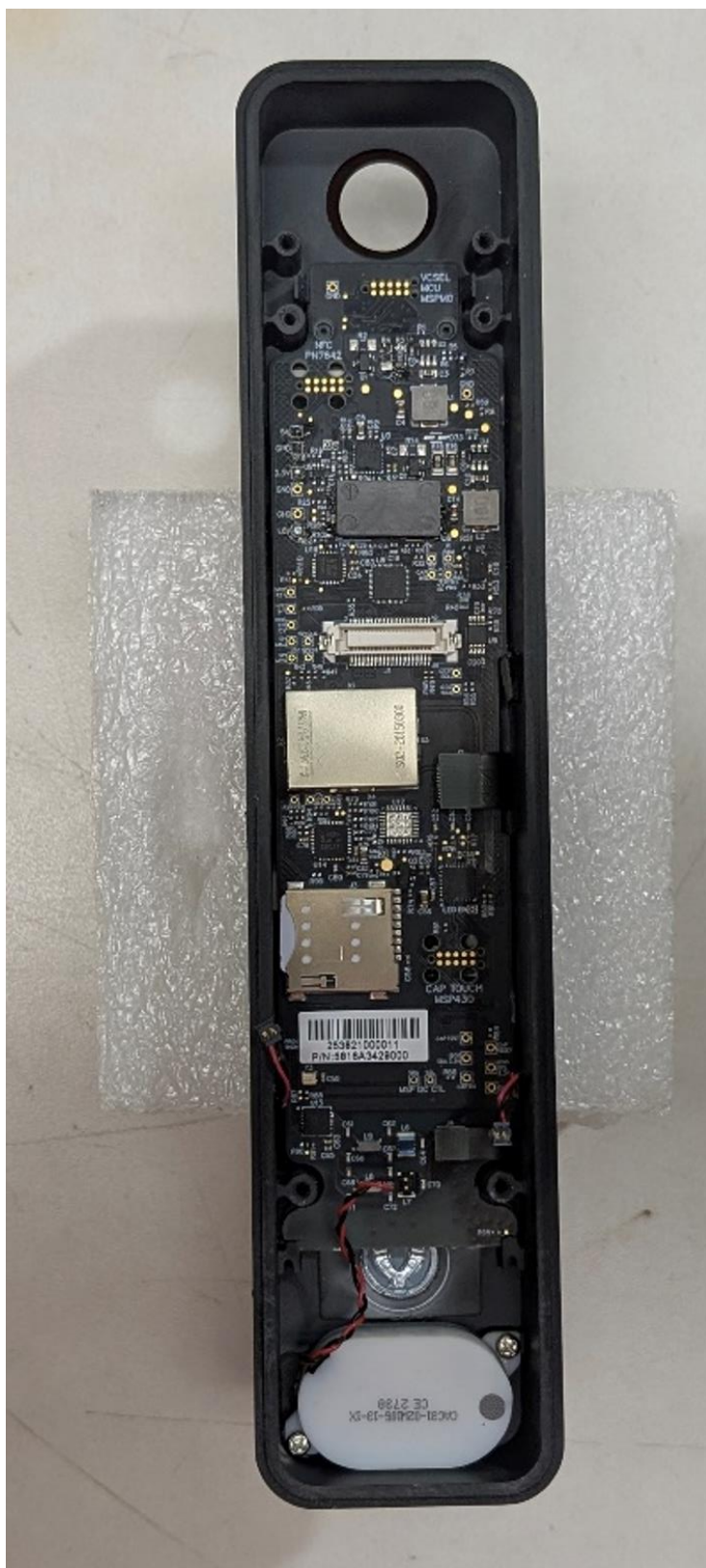
Photograph 13 – Front Housing with Keypad PCB Installed on top of NFC Antenna
