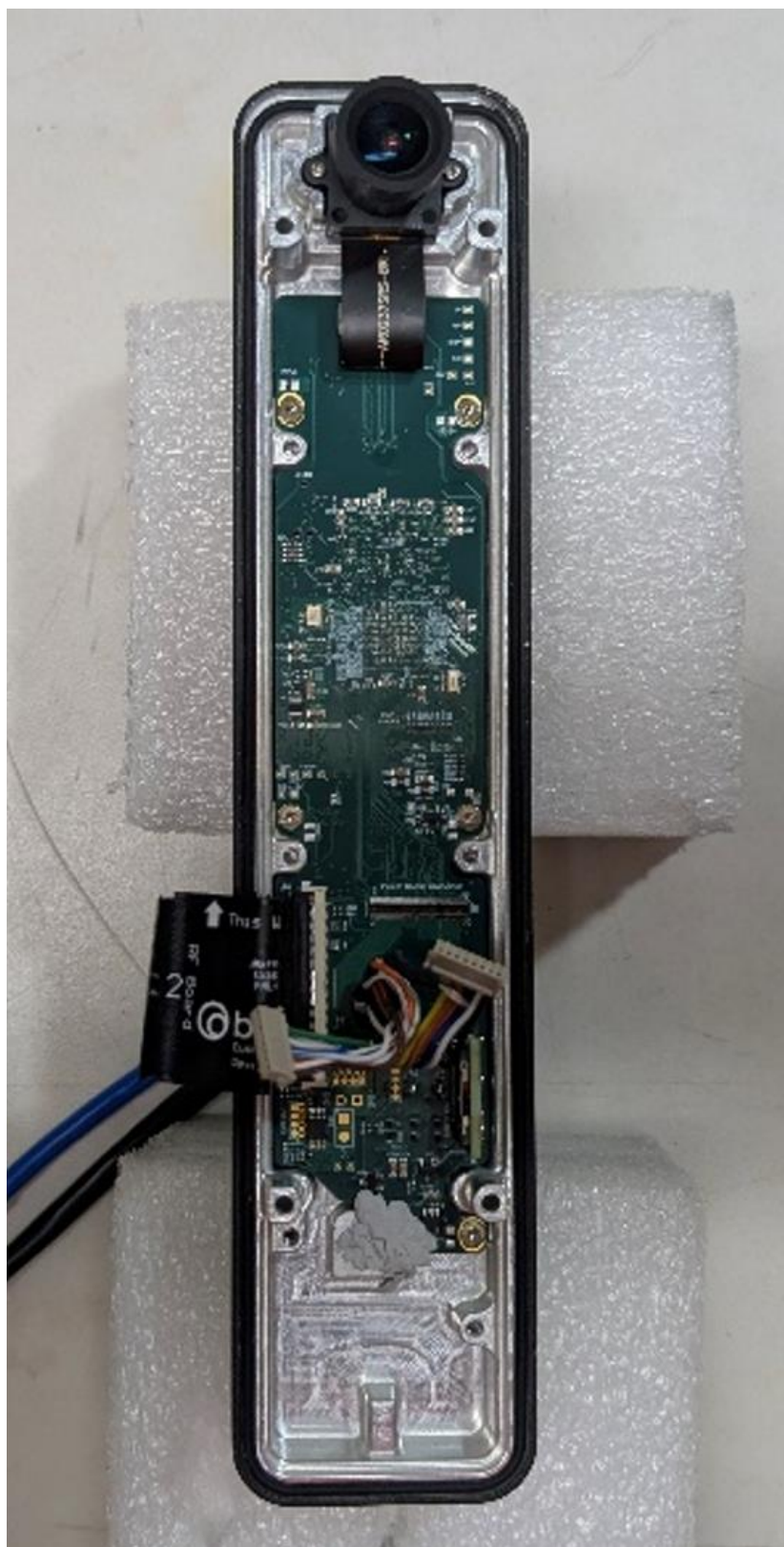
Photograph 15 – Back Housing with Main PCB
