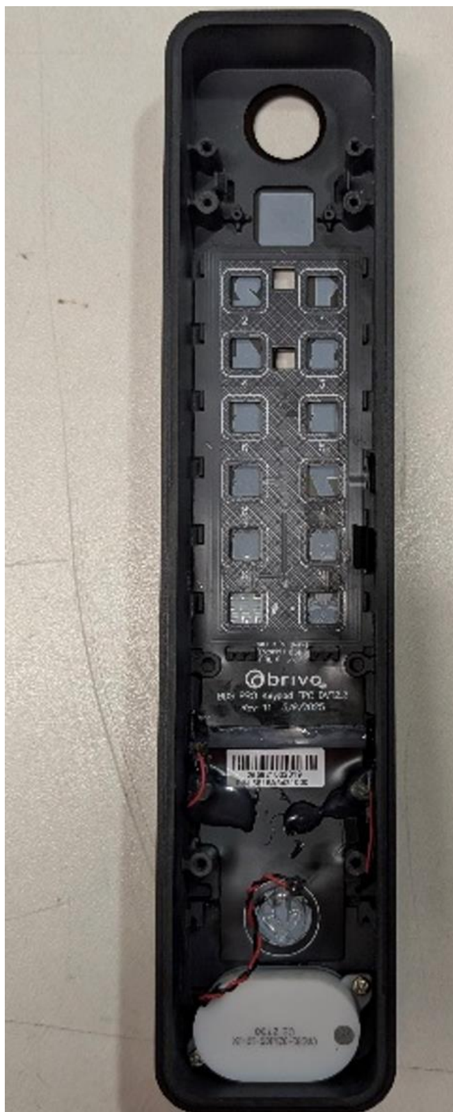
Photograph 12 – Front housing with NFC antenna in place
