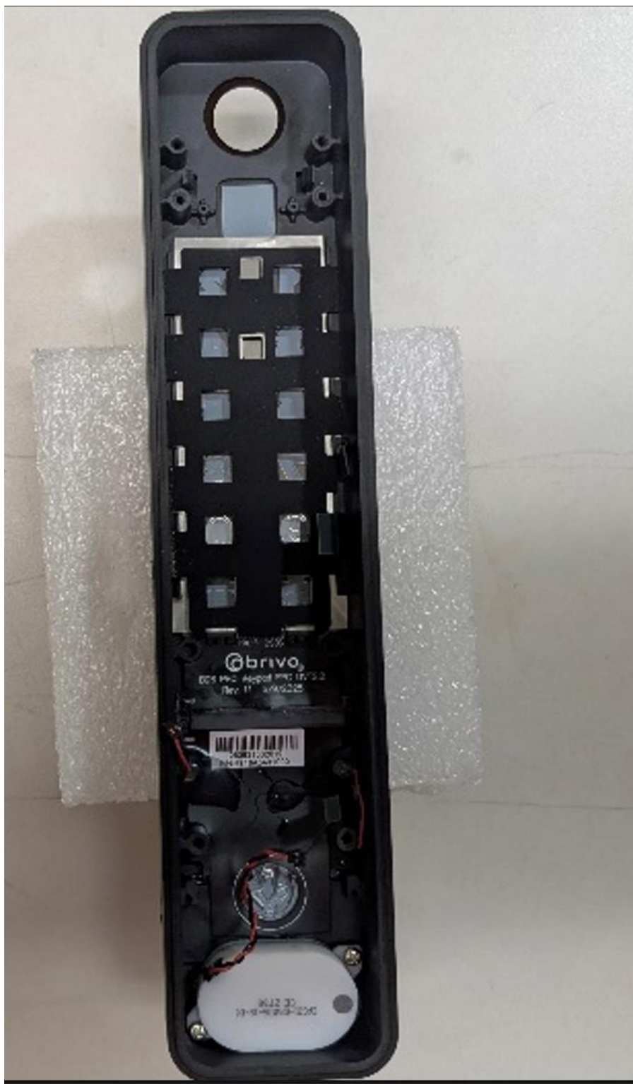
Photograph 11 – Front Housing with all PCBs removed, Front Keypad overlay visible.
