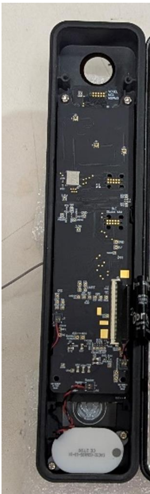
Photograph 14 – Front housing with RF Board on top of Keypad PCB
