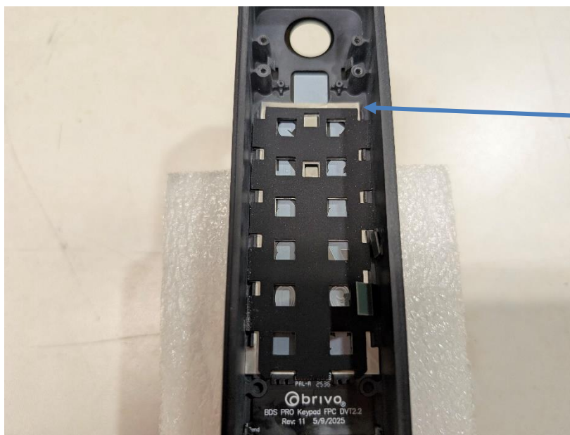
Photograph 18: Close-up of Keypad with RF Shielding
