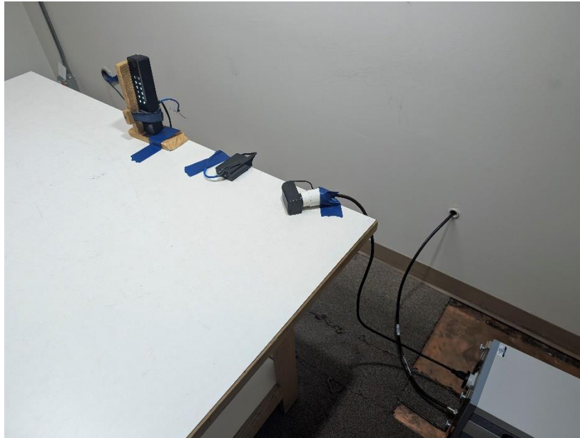
Photograph 5: Front View Conducted Emissions Worst Case Configuration
