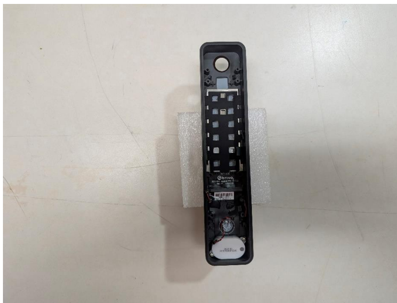
Photograph 17: Enclosure Front with Keypad Board Removed
