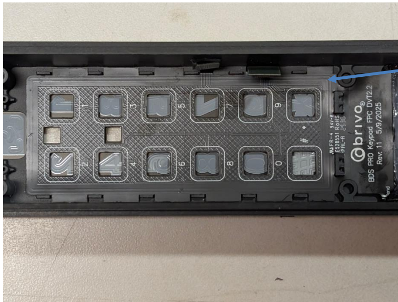
Photograph 20: Closeup View of Enclosure with RF Shielding Removed from Keypad, Showing NFC Antenna
