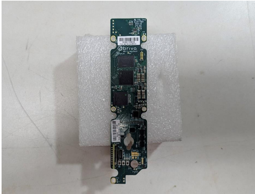
Photograph 43: Back of PCB "Main Board"
