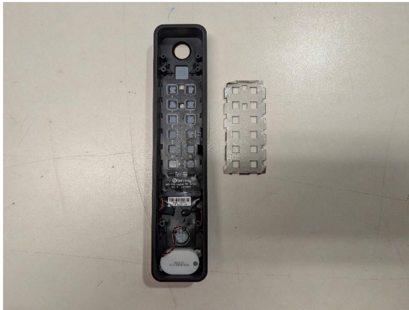
Photograph 19: Enclosure with RF Shielding Removed from Keypad
