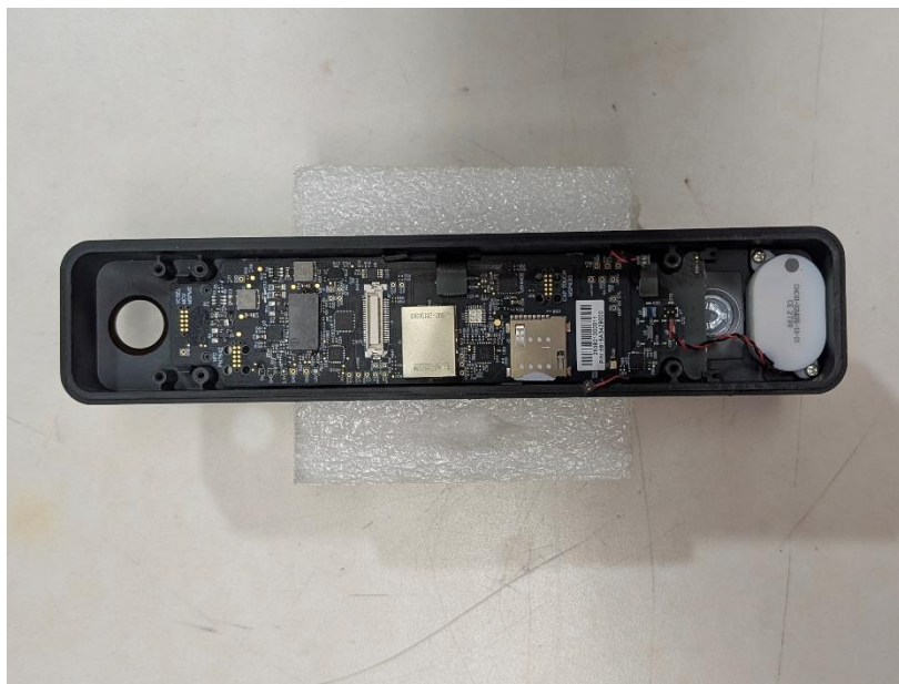
Photograph 16: Enclosure Front with “Keypad Board”
