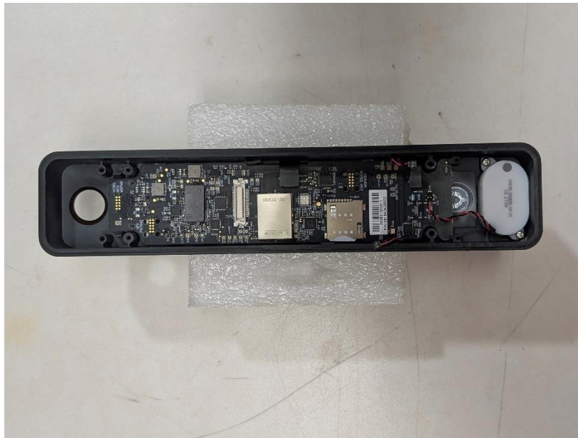
Photograph 11: Enclosure Front with "Keypad Board"
