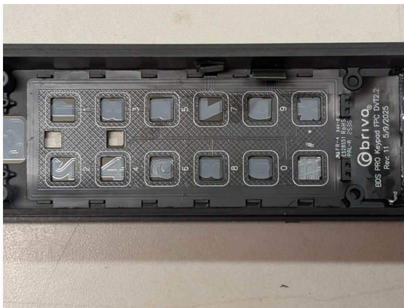
Photograph 15: Closeup View of Enclosure with RF Shielding Removed from Keypad, Showing NFC Antenna
