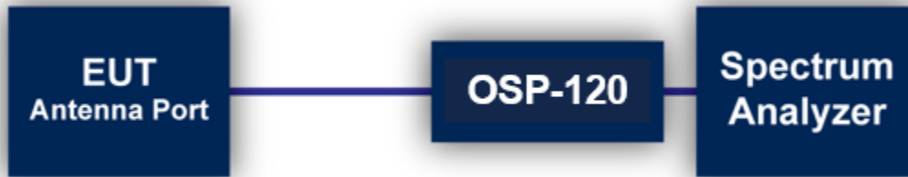
Figure 2: Direct Connection at the Antenna Port Test
