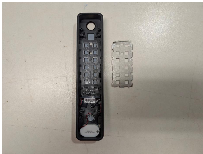
Photograph 14: Enclosure with RF Shielding Removed from Keypad
