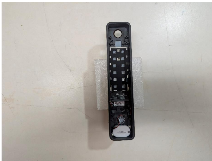
Photograph 12: Enclosure Front with Keypad Board Removed
