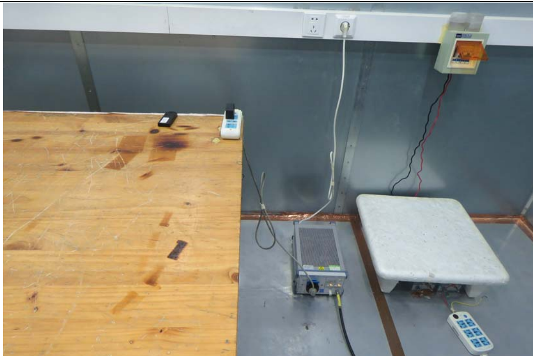
Picture 2: Conducted Emissions Test Setup
