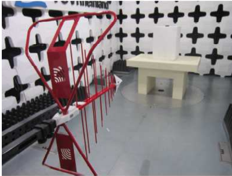
RADIATED TEST SETUP FCC 15 – RSS247
